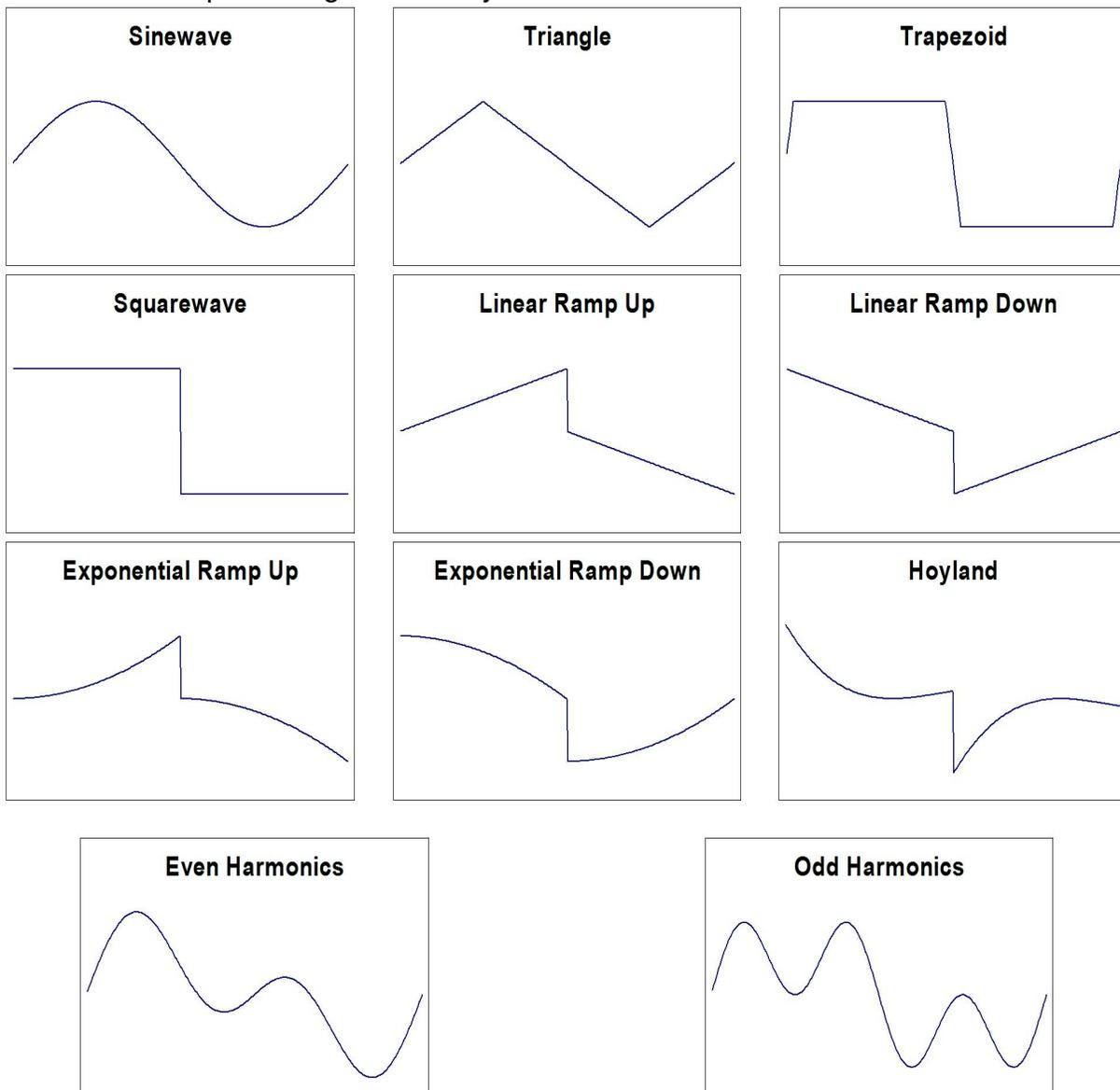
**“Harmonics”** are all of those Sinewaves of different frequencies that make up a complex waveform, such as Triangle, Square, and all others. Here is a list of “Harmonic Content” of the Power waveforms generated by the Ultra.
