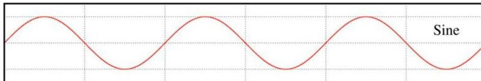
Mapping the elevation of a point on the perimeter of a circle as it constantly turns can show a Sinewave.
